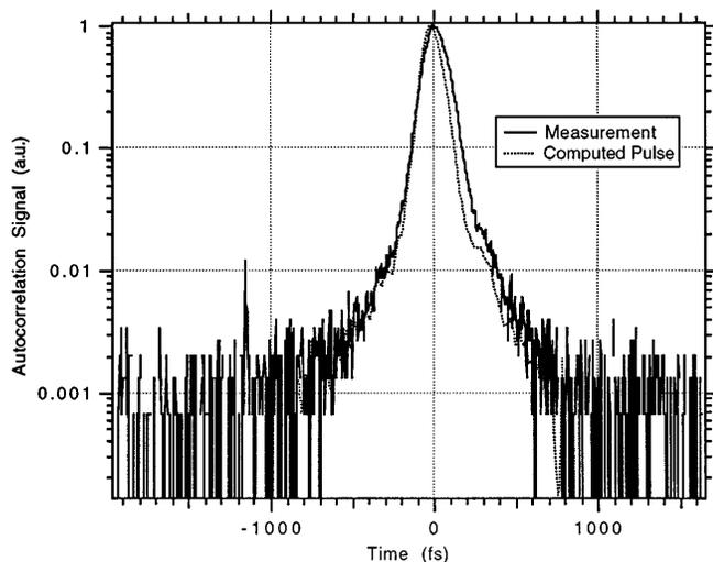
Fig. 2. Single-shot third-order autocorrelation of the full-energy laser beam. Also shown is a computed pulse shape based on the pulse measurement. This pulse duration is 120 fs FWHM. This value is in excellent agreement with that obtained when a Gaussian pulse shape is assumed.
