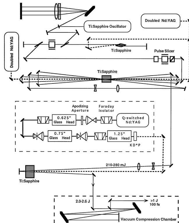
Fig. 1. Diagram of the laser system including the frequency-doubled Nd:glass laser used to pump the third amplifier (1 in. = 2.54 cm).
