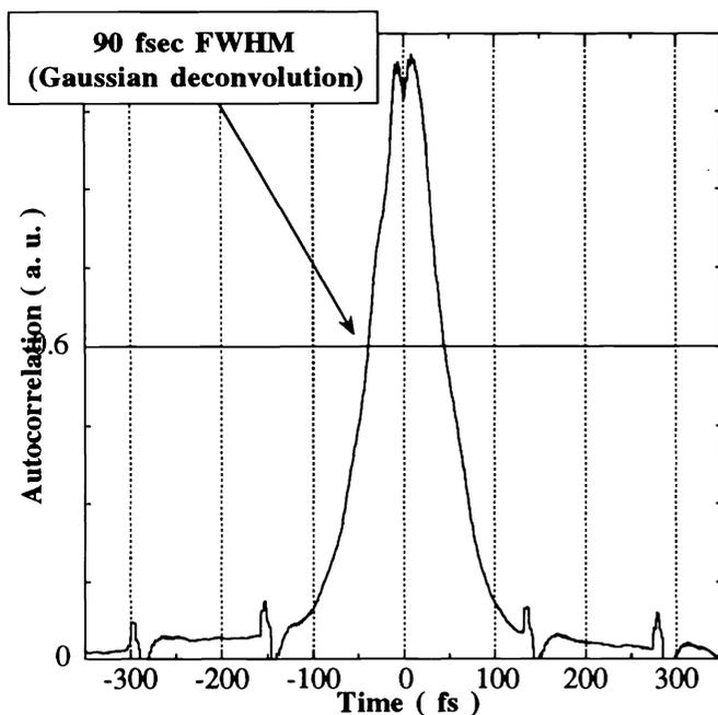
Fig. 6. Second order autocorrelation of the 250 mJ amplified pulse (assuming Gaussian deconvolution).
