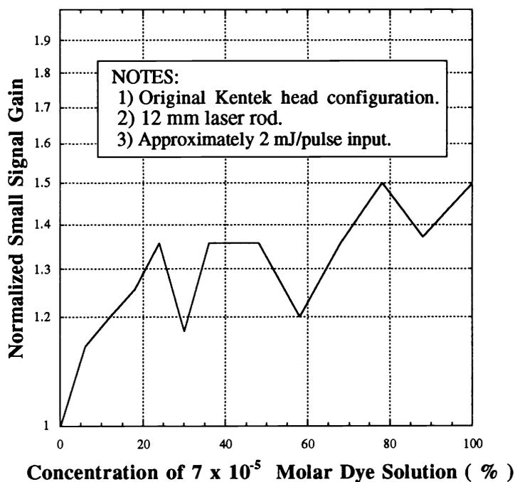
Figure 3 demonstrates the effect of adding LD-489 laser dye to the amplifier head. As shown, the addition of the UV converting dye in the pump chamber improves the peak small signal gain by 50%.
