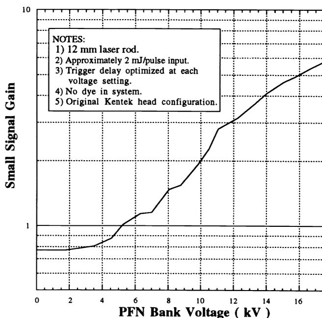
Fig. 2. Small signal gain of the CRD-4 amplifier as a function of PFN voltage.
