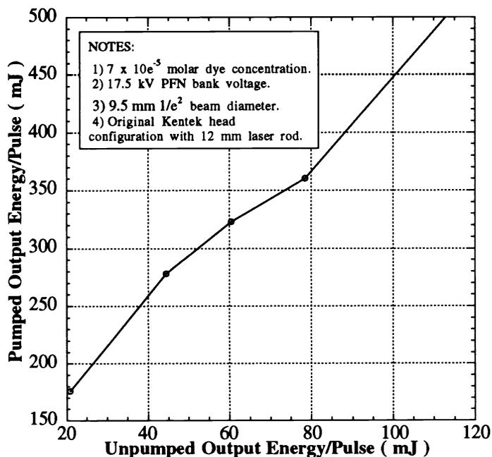
Fig. 4. Transmitted energies through the amplifier with and without pumping.
