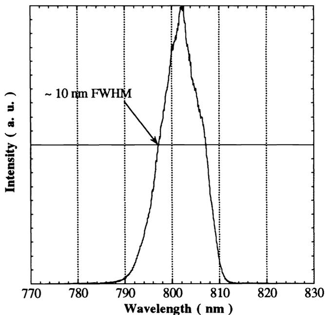
Fig. 5. Spectrum of the 250 mJ, 90 fsec compressed pulse.
