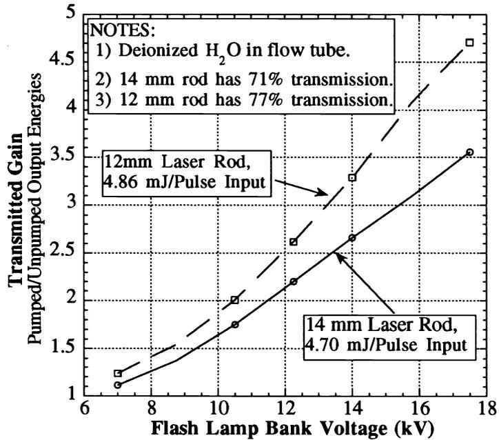
Fig. 8. Pumped/unpumped transmitted small signal gain as a function of the amplifier pulse forming network voltage.
