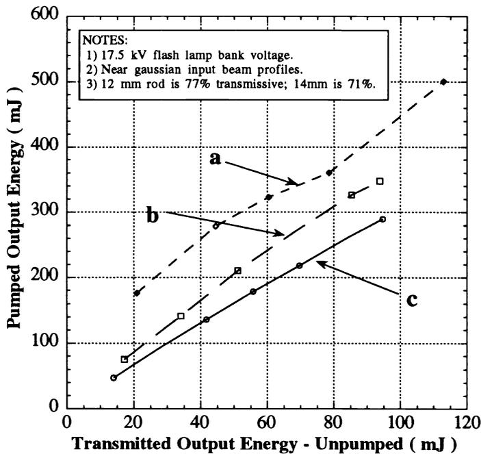
Fig. 9. High energy amplification: a) 12 mm rod in original configuration using KC-331 flow tube and LD-489 laser dye; b) 12 mm rod in modified head configuration with KTF-2 flow tube; c) 14 mm rod in modified head.
